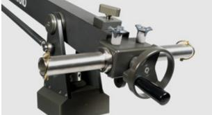
Its counterweight arm can be steplessly adjusted by a crank and extended up to a max. of 100 cm. A userfriendly brake attached to the end of the GF-Mini Jib also serves as friction, depending on the tight-ening torque. Most Jib Arm components are made of aluminium and have a very hard and durable surface protection [Hart-Coat®].
