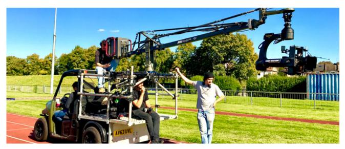
The GF-Multi Jib is a professional, lightweight and modular Jib arm, suitable for carrying all general remote head systems. It is portable, mobile and mounts on most standard dollies fitted with Euro-adapter or Mitchell mounts.
